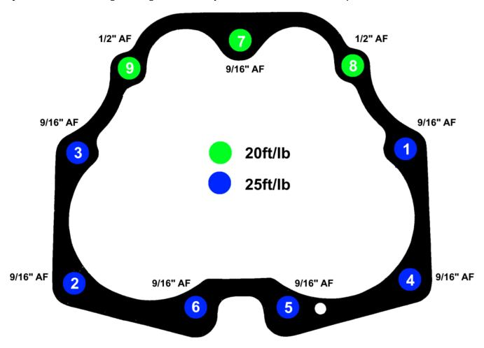
Cylinder Base 850 Tightening Order, Torque, and Wrench Size:
