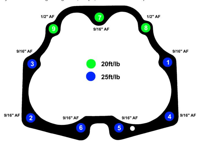
Cylinder Base 850 Tightening Order, Torque, and Wrench Size:
